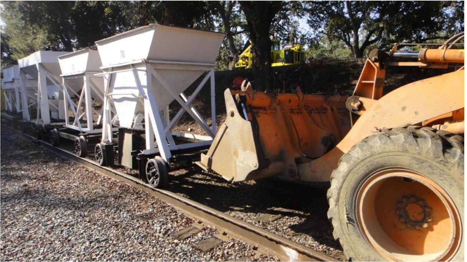
Mike F. brings in the loader to act as an anchor to block the other three full ballast cars from running-away down the hill
